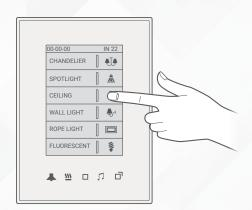
Test by pressing on the wall panel's 3>> ON/OFF button. The module relay should respond by turning ON and OFF accordingly.
