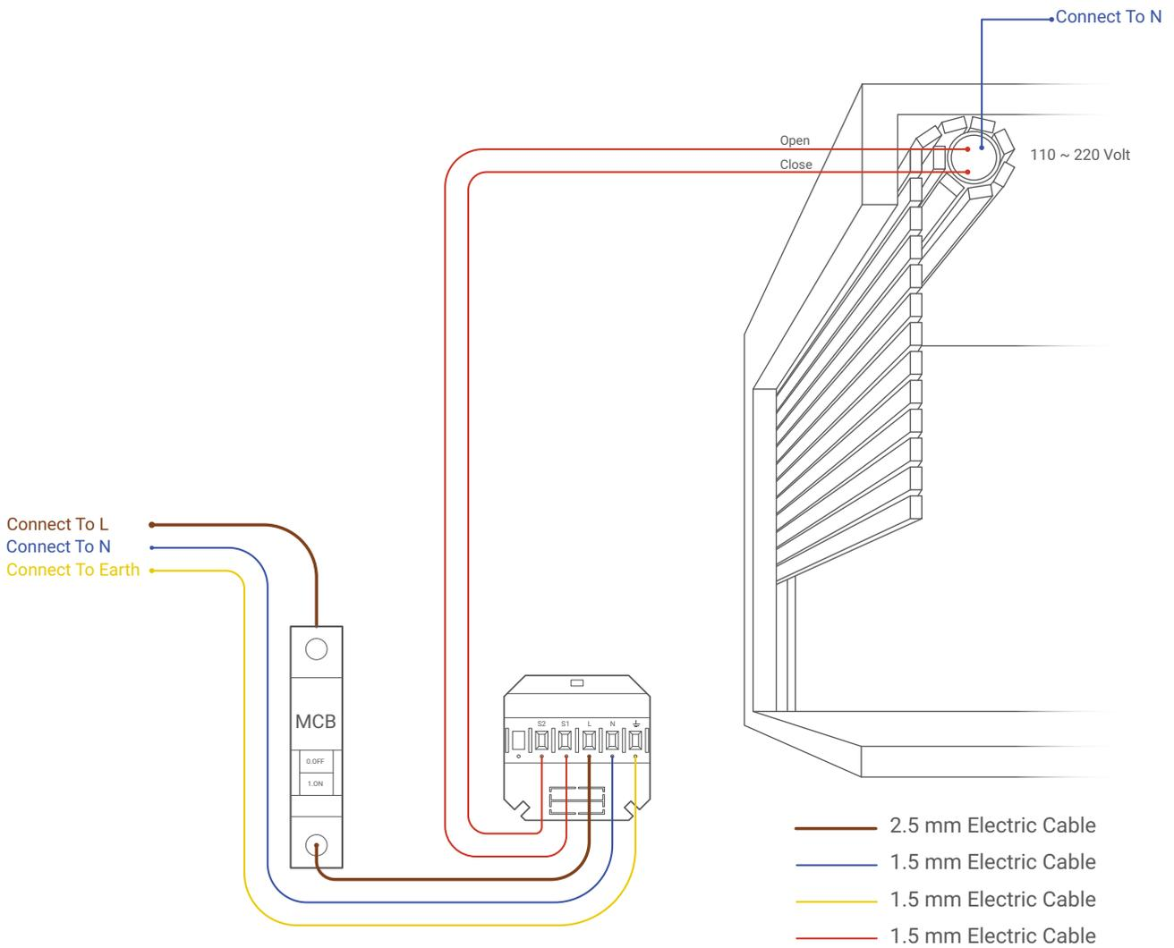
▲ Figure 2: Motors Connection Diagram
