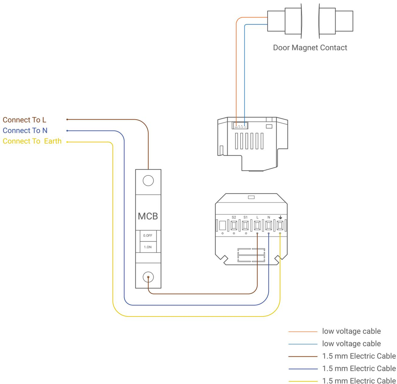
▲ Figure 3: Magnetic Door Contact Connection Diagram
