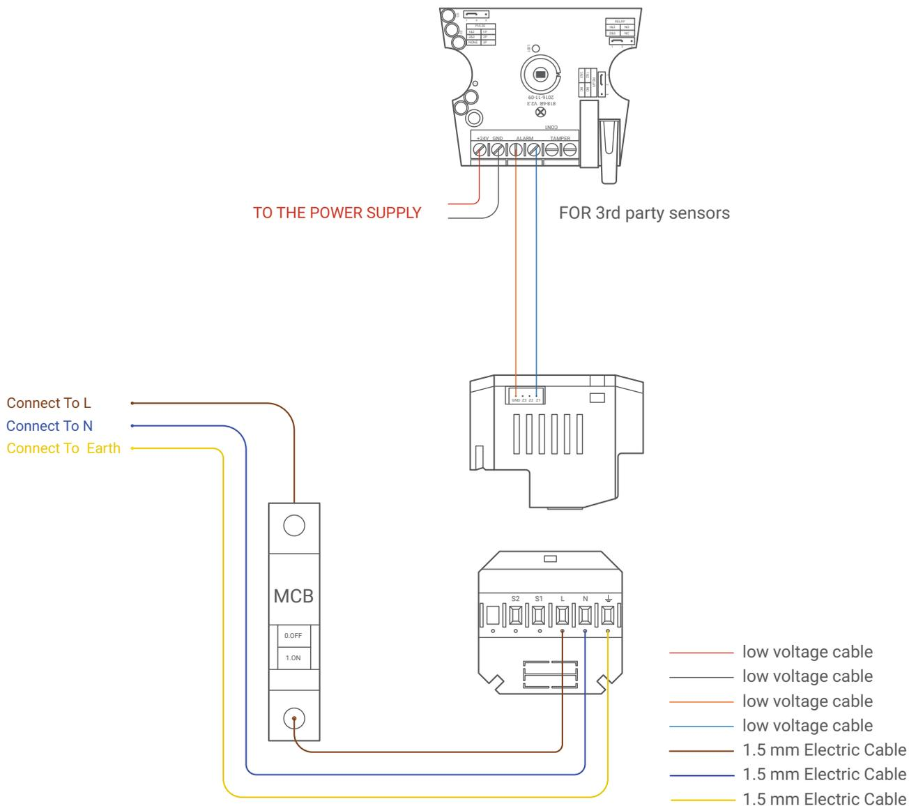
▲ Figure 4: 3<sup>rd</sup> Party Sensor Connection Diagram
