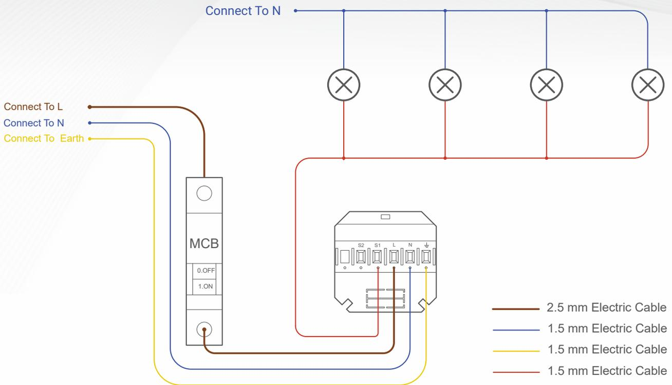
▲ Figure 1: Lights Connection Diagram
