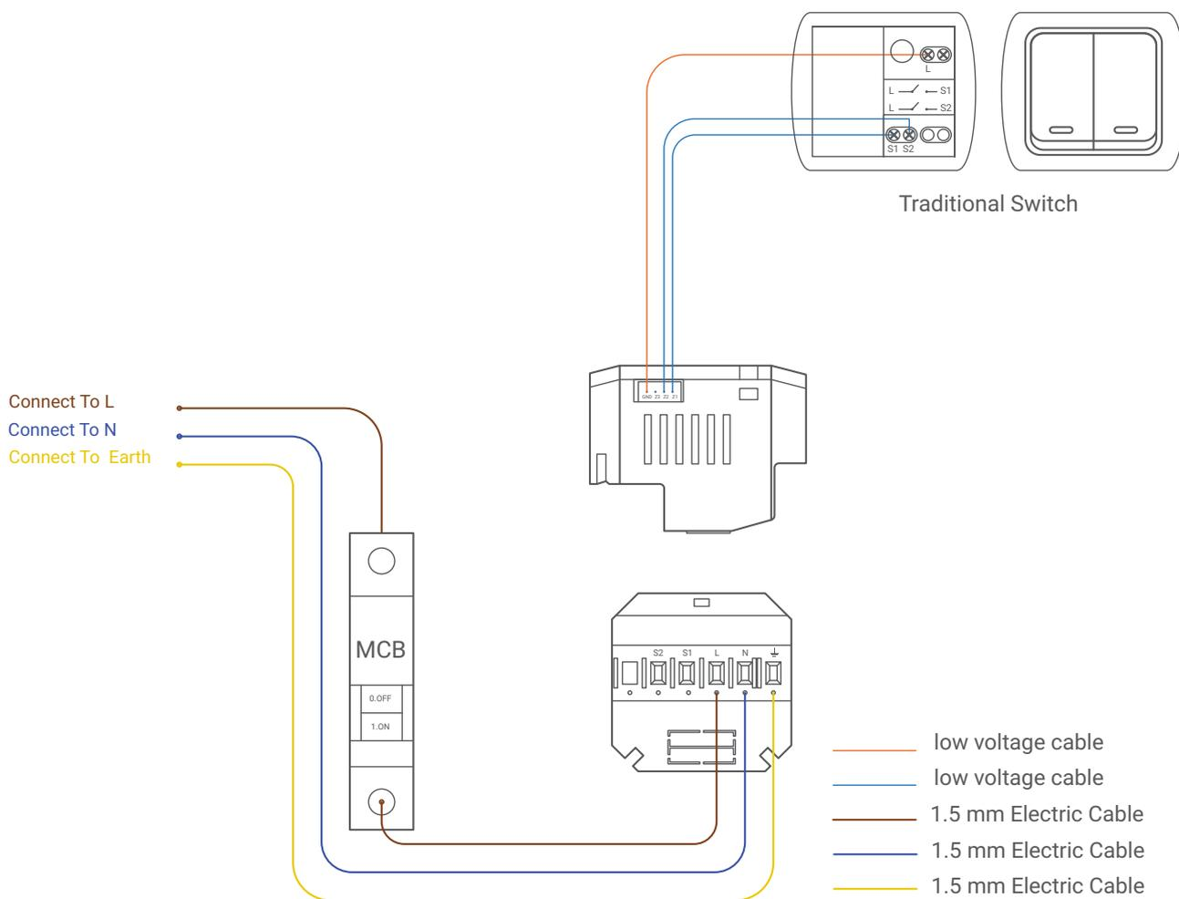
▲ Figure 5: Traditional Switch Connection Diagram
