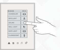
**3** Test by pressing on the wall panel's ON/OFF button. The module relay should respond by turning ON and OFF accordingly.
