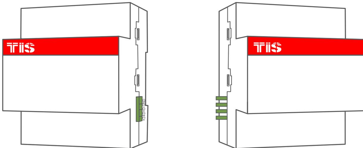
▲ Figure 2: DIN-Rail BUS Module Configuration Diagram
