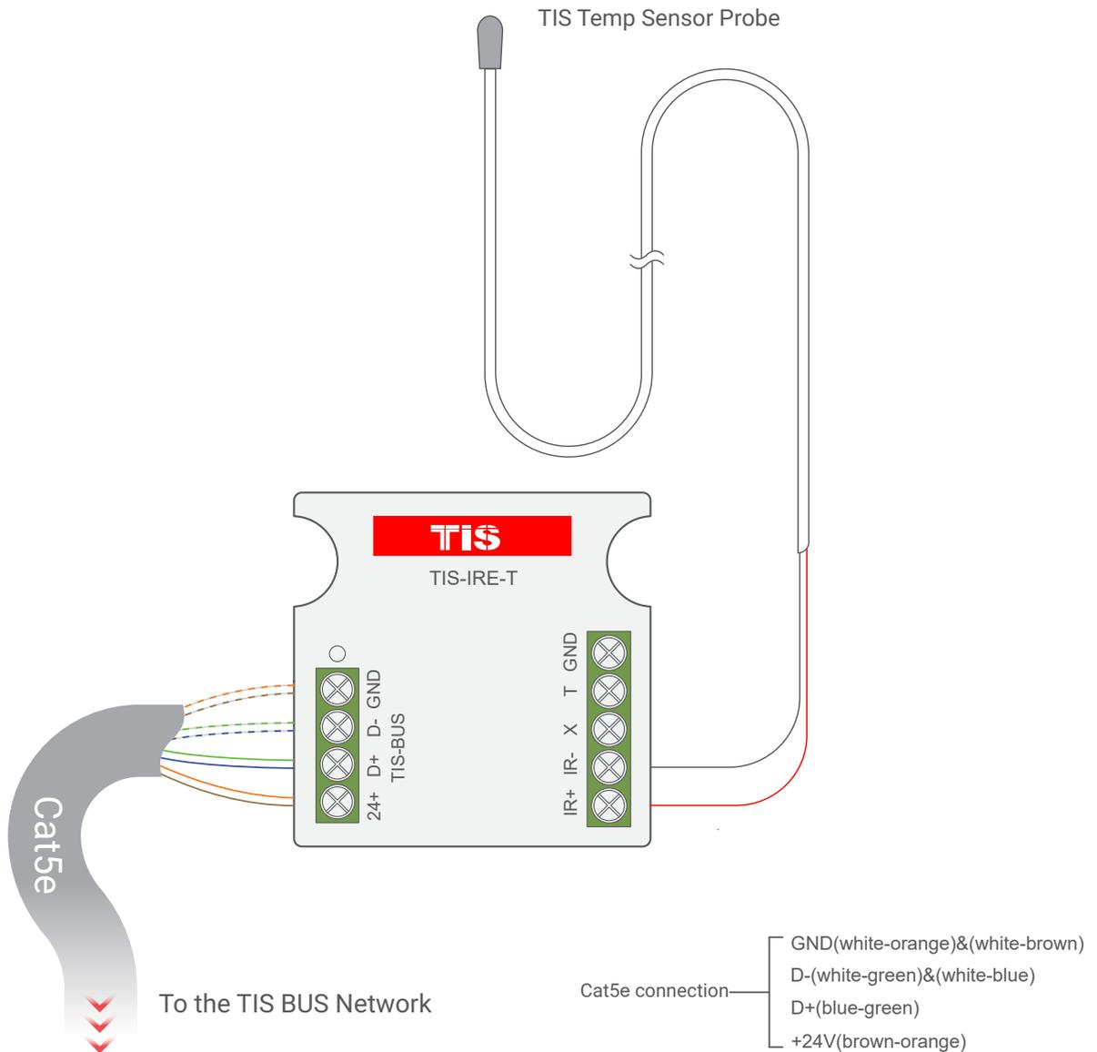
▲ Figure 2: TIS Temperature probe Connection Diagram
