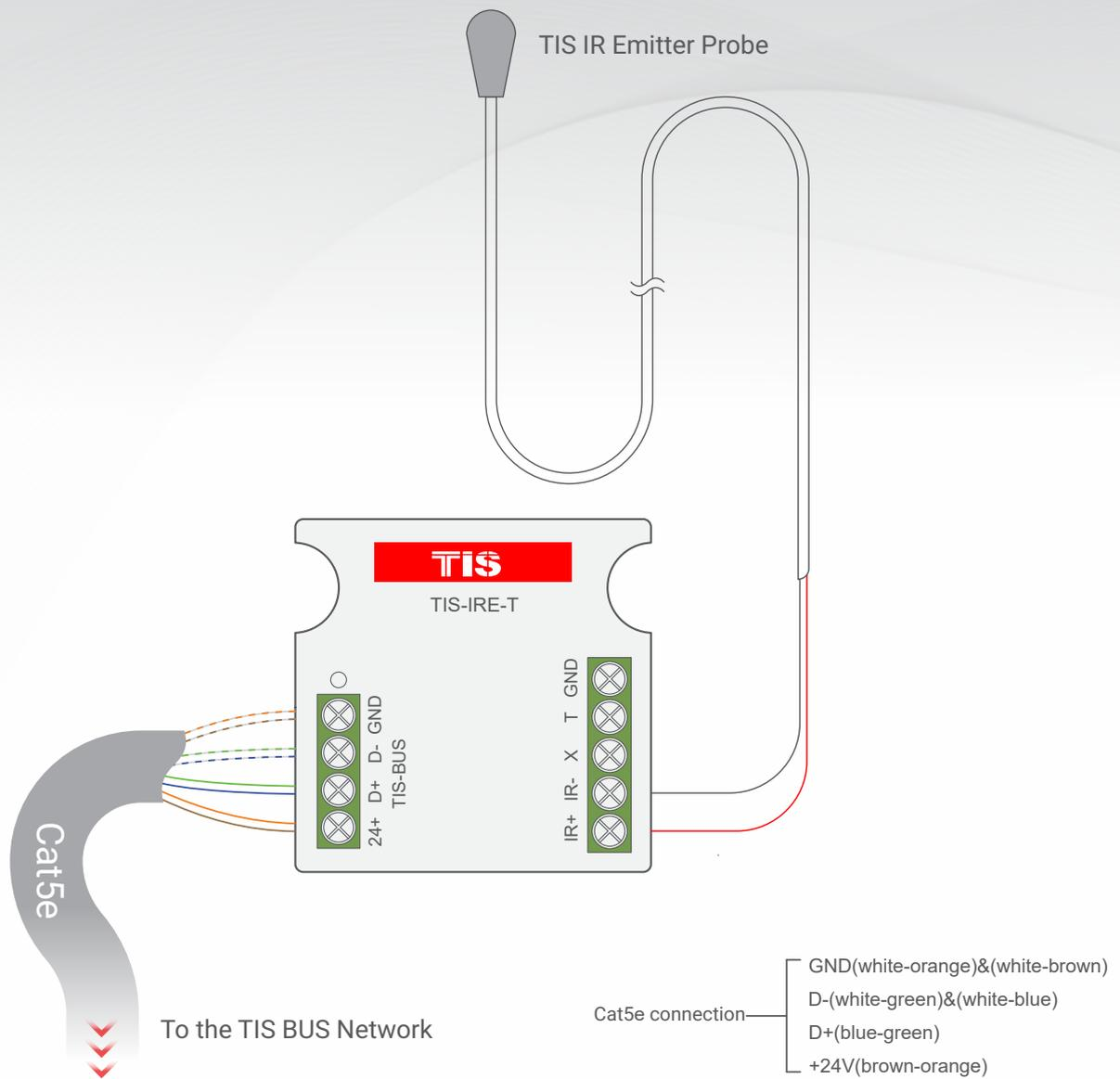
▲ Figure 1: TIS IR Emitter probe Connection Diagram
