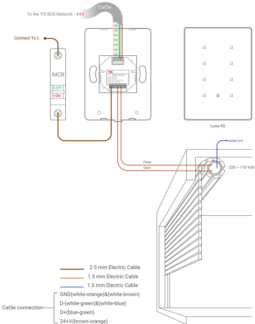
▲ Figure 3: Luna 9G & ADD-3R-5A Motors Connection Diagram
