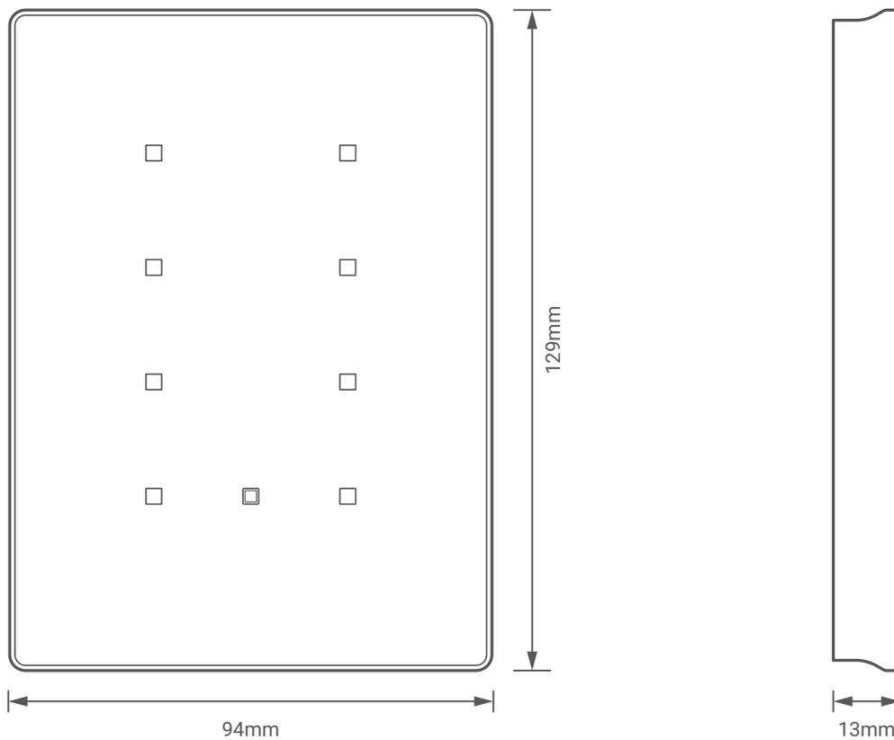
▲ Figure 14: Module's Dimension Diagram
