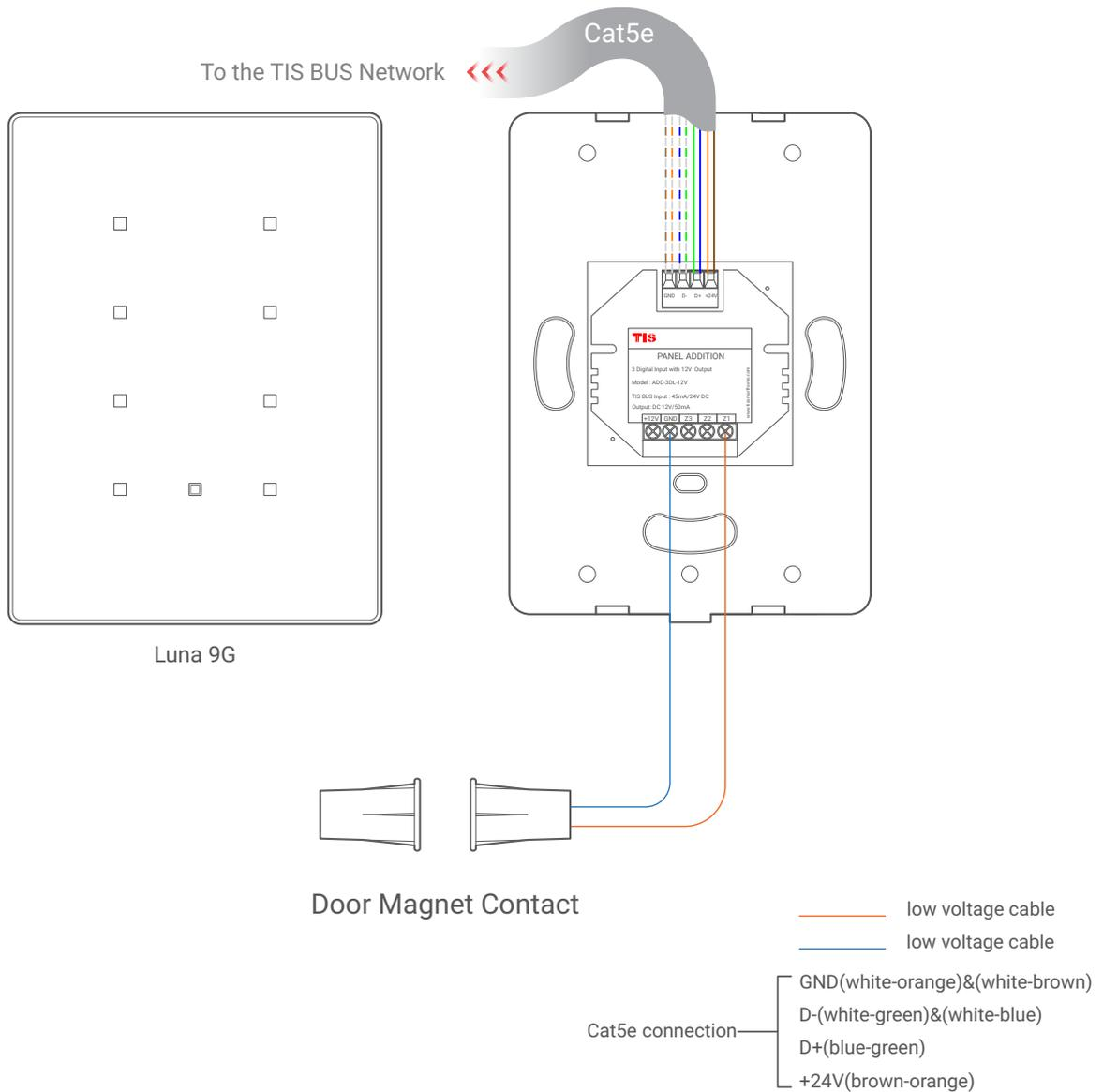
▲ Figure 5: Luna 9G & ADD-3DL-12V Magnetic Door Contact Connection Diagram
