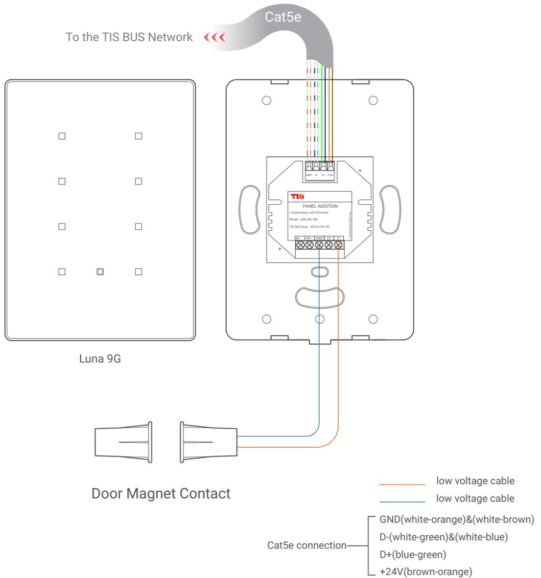
▲ Figure 11: Luna 9G & ADD-2DL-IRE Magnetic Door Contact Connection Diagram
