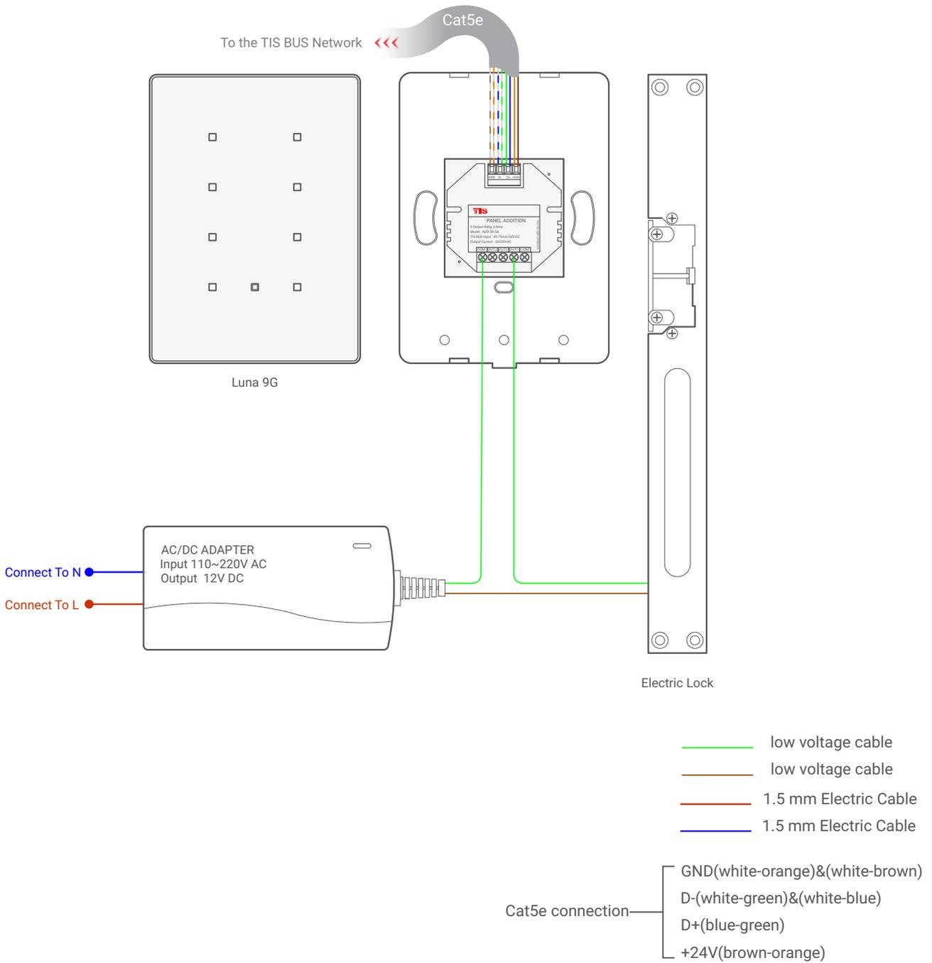
▲ Figure 4: Luna 9G & ADD-3R-5A Electric Lock Connection Diagram
