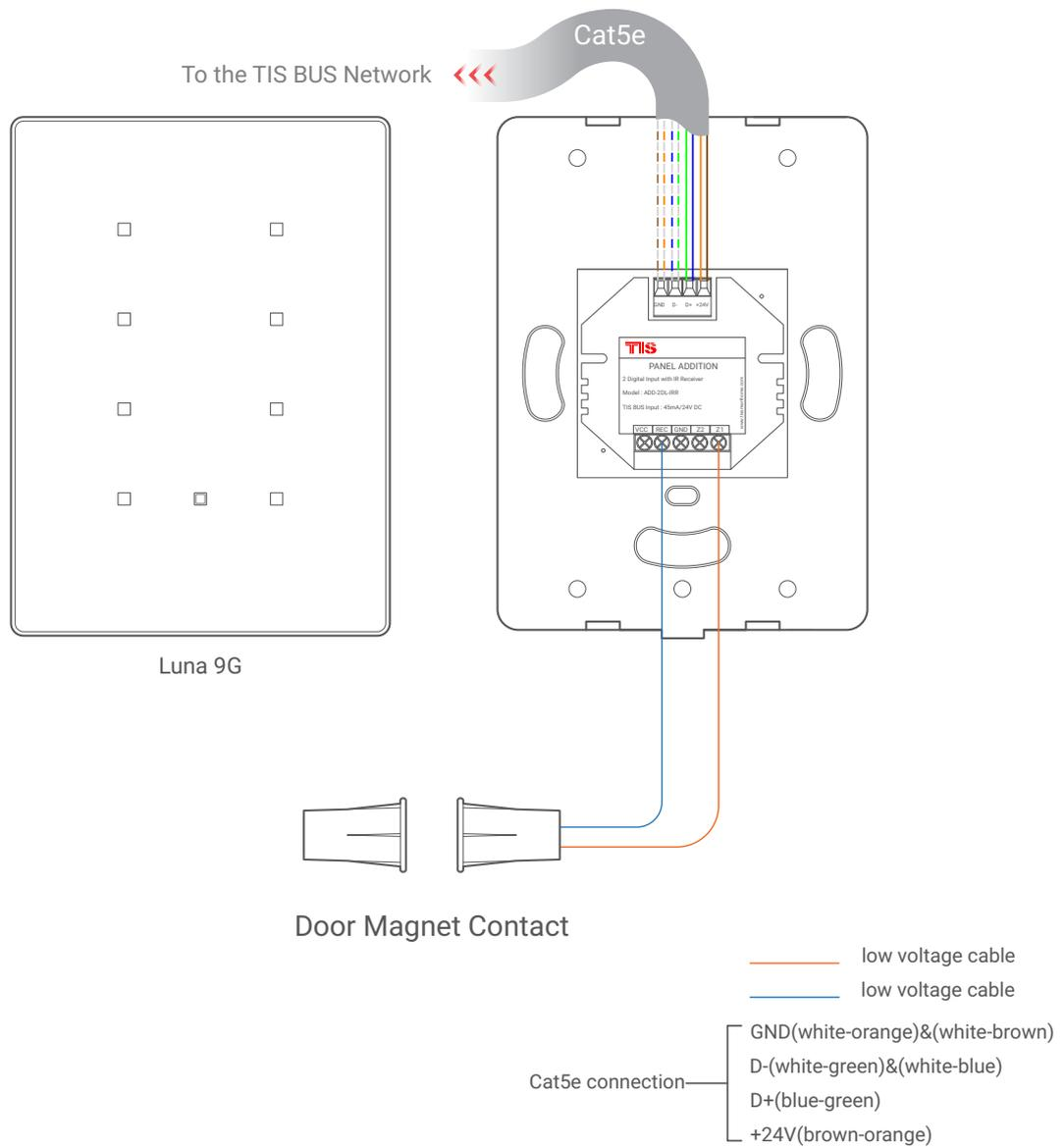
▲ Figure 8: Luna 9G & ADD-2DL-IRR Magnetic Door Contact Connection Diagram
