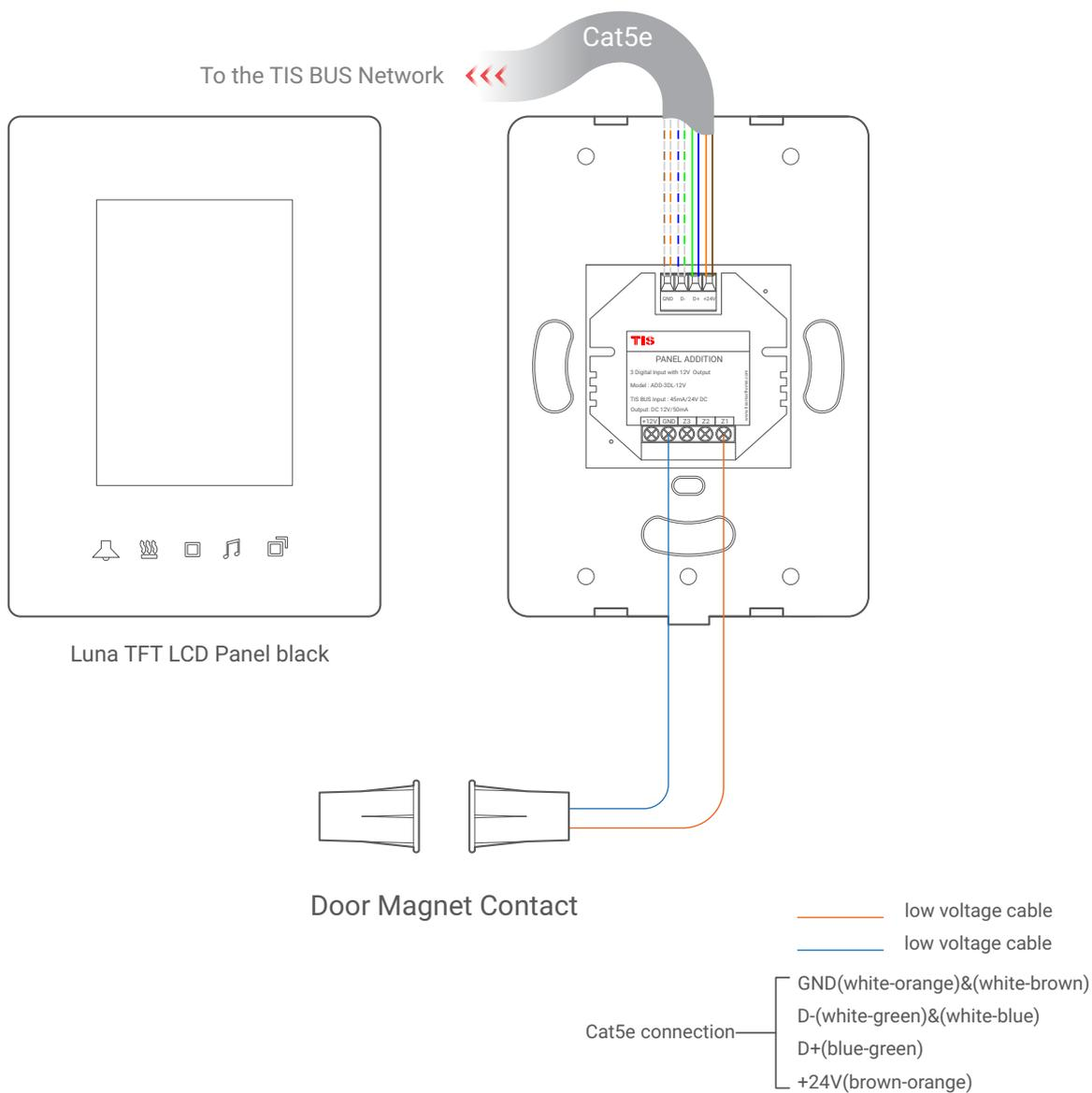
▲ Figure 5: Luna TFT & ADD-3DL-12V Magnetic Door Contact Connection Diagram
