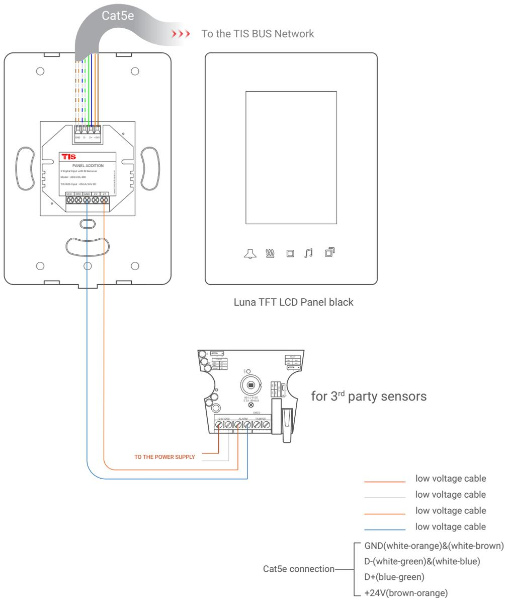
▲ Figure 9: Luna TFT & ADD-2DL-IRR 3<sup>rd</sup> Party Sensor Connection Diagram
