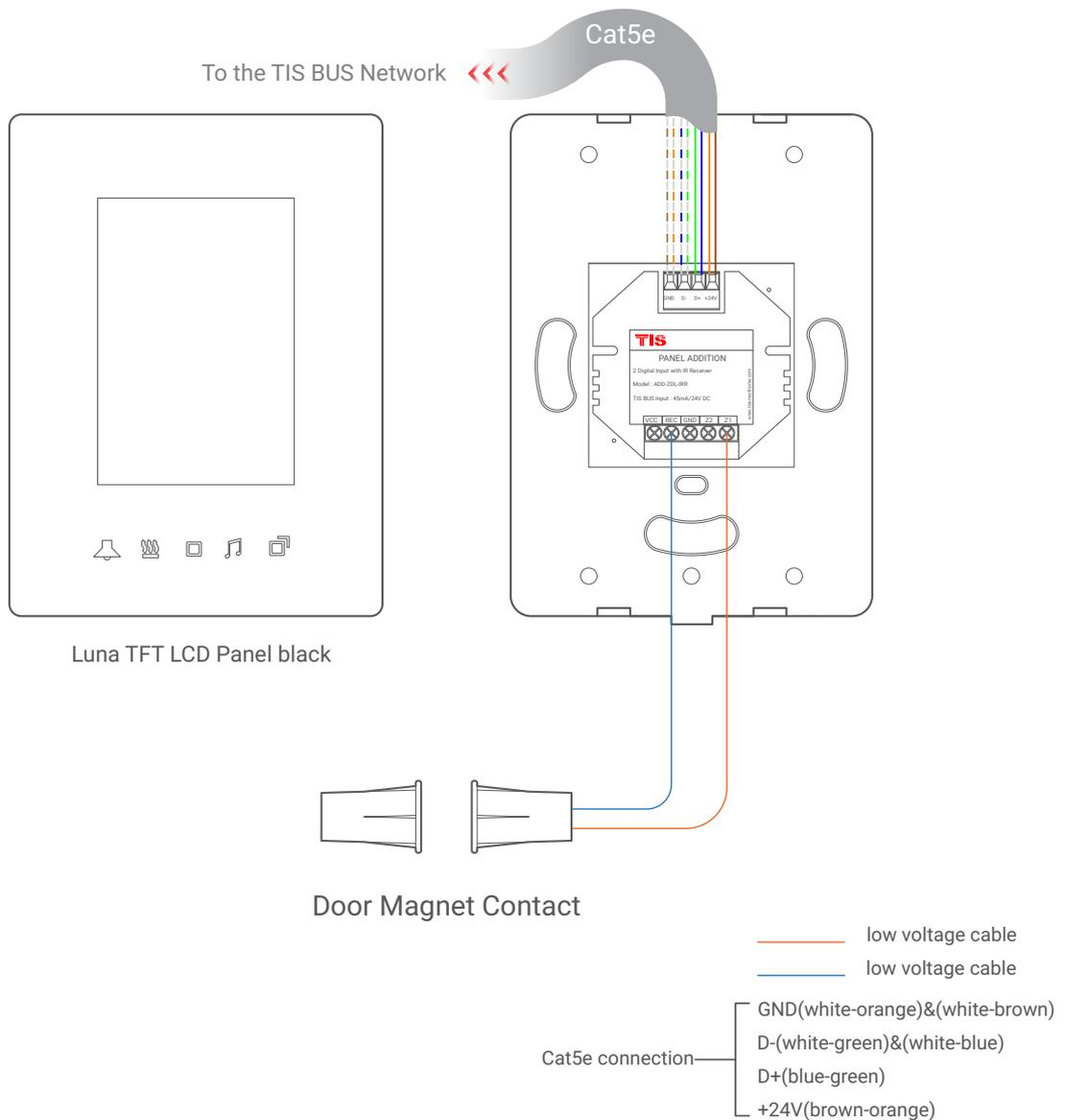
▲ Figure 8: Luna TFT & ADD-2DL-IRR Magnetic Door Contact Connection Diagram
