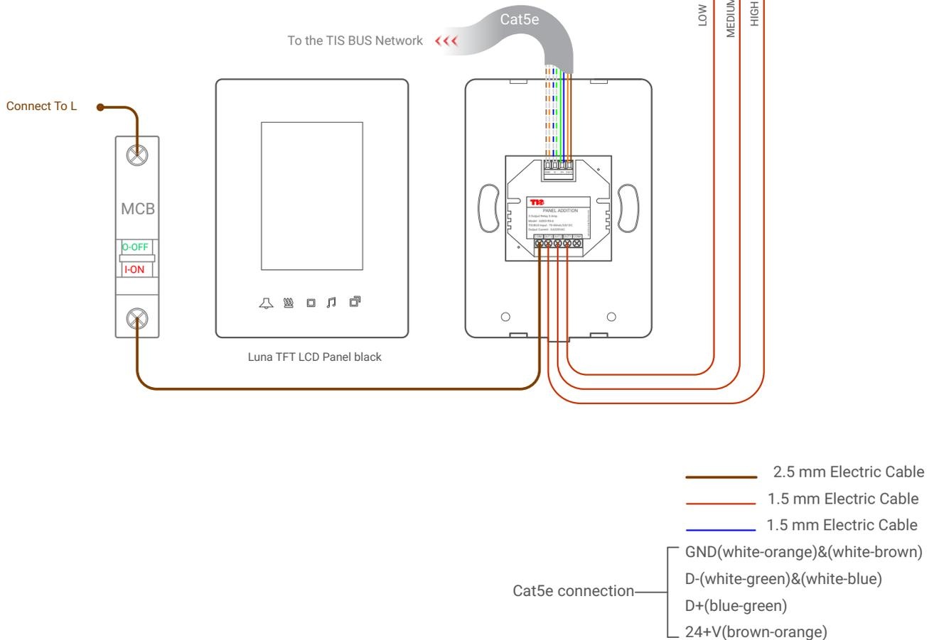
▲ Figure 2: Luna TFT & ADD-3R-5A FCU Connection Diagram
