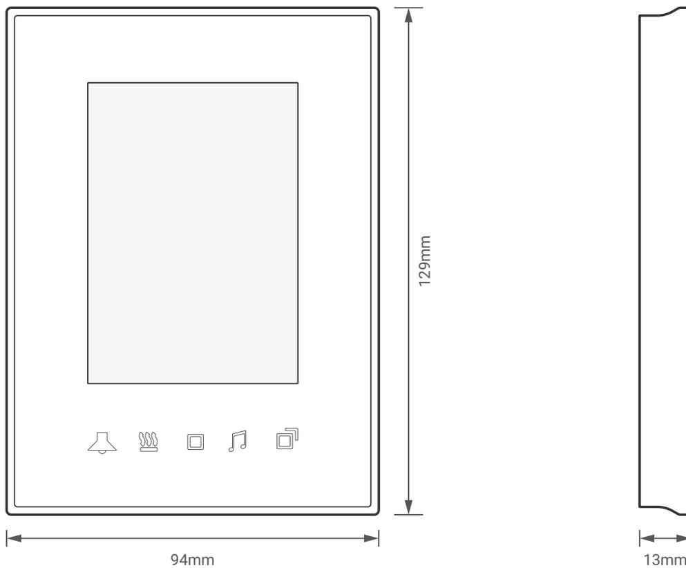
▲ Figure 14: Module's Dimension Diagram
