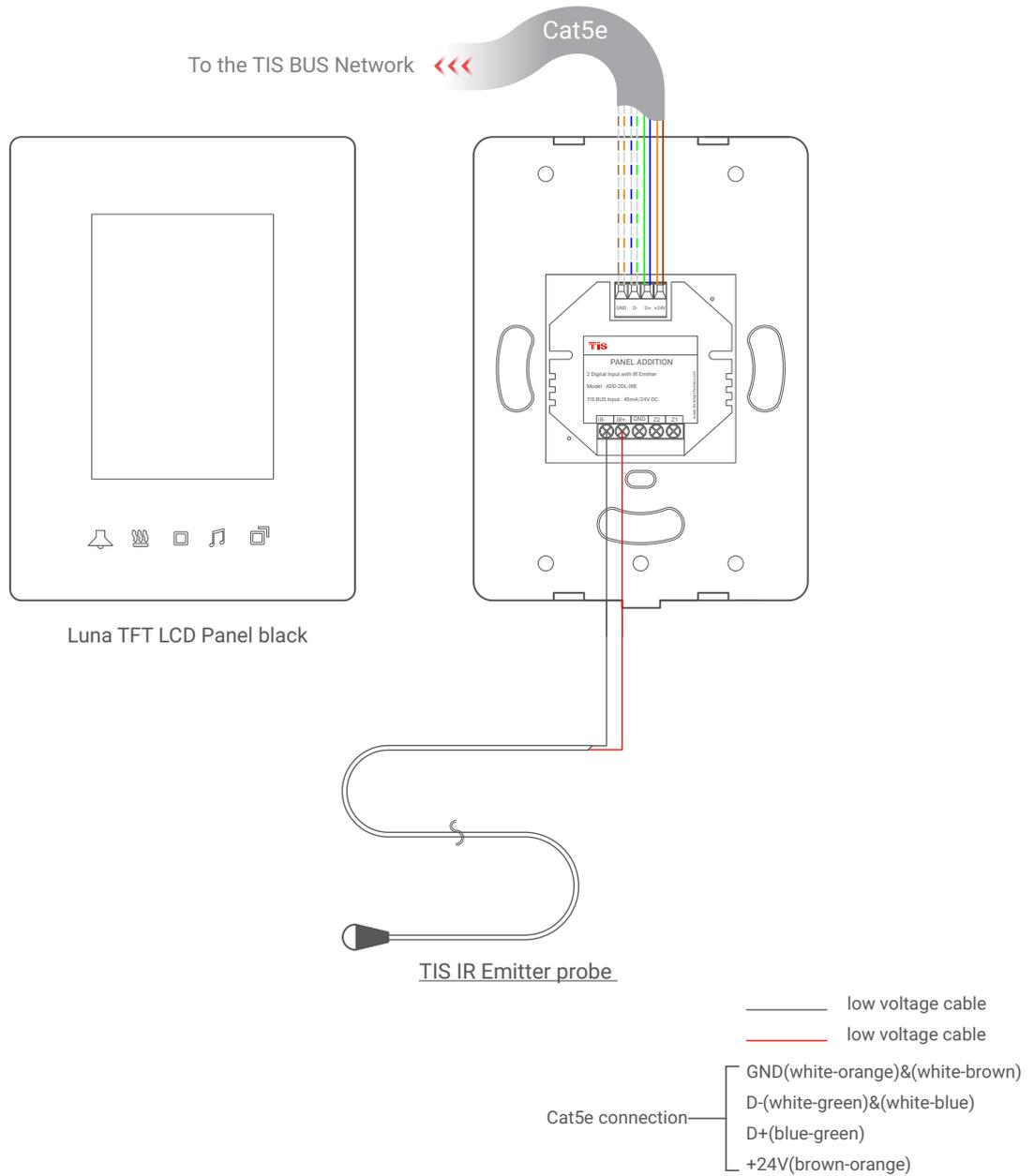
▲ Figure 10: Luna TFT & ADD-2DL-IRE Connection Diagram
