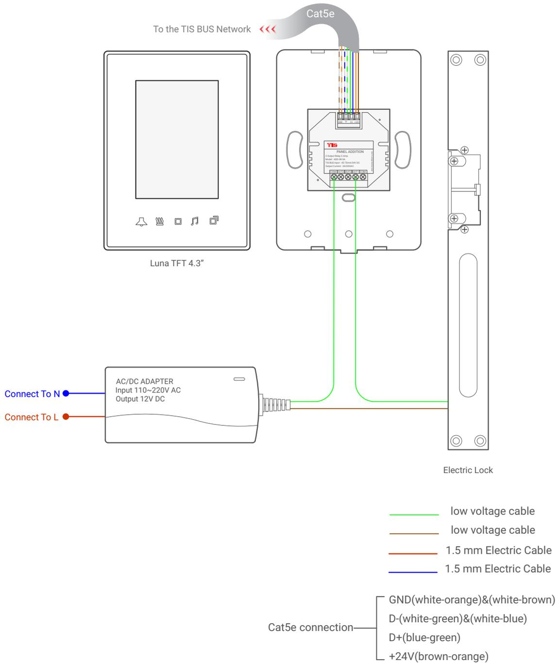
▲ Figure 4: Luna TFT & ADD-3R-5A Electric Lock Connection Diagram
