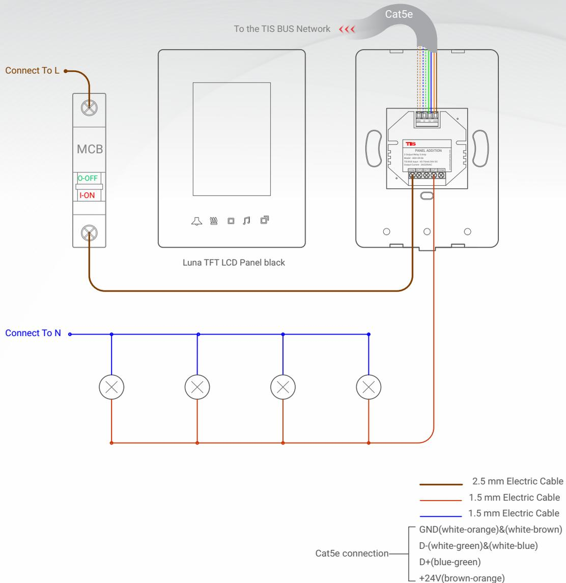
▲ Figure 1: Luna TFT & ADD-3R-5A Lights Connection Diagram
