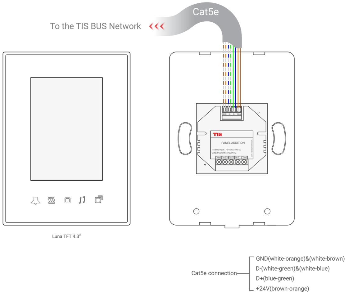
▲ Figure 13: Luna TFT Bus Connection Color Coding
