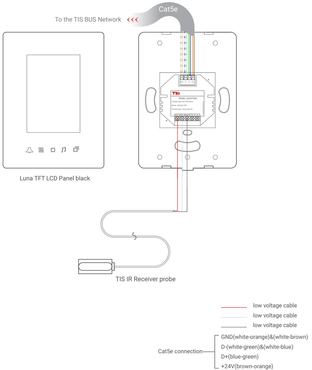
▲ Figure 7: Luna TFT & ADD-2DL-IRR Connection Diagram
