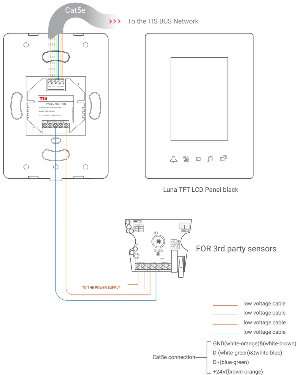
▲ Figure 12: Luna TFT & ADD-2DL-IRE 3<sup>rd</sup> Party Sensor Connection Diagram
