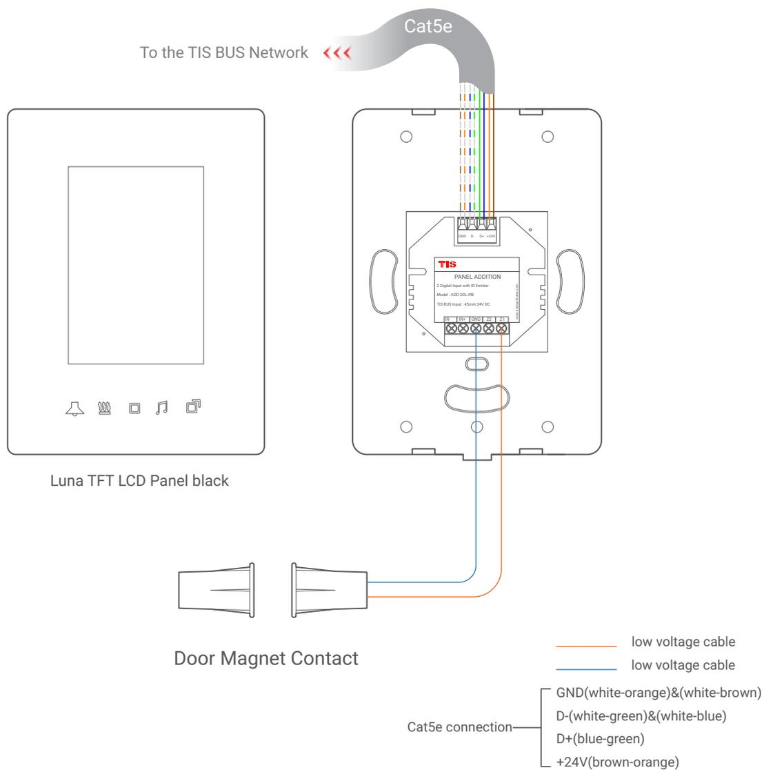
▲ Figure 11: Luna TFT & ADD-2DL-IRE Magnetic Door Contact Connection Diagram
