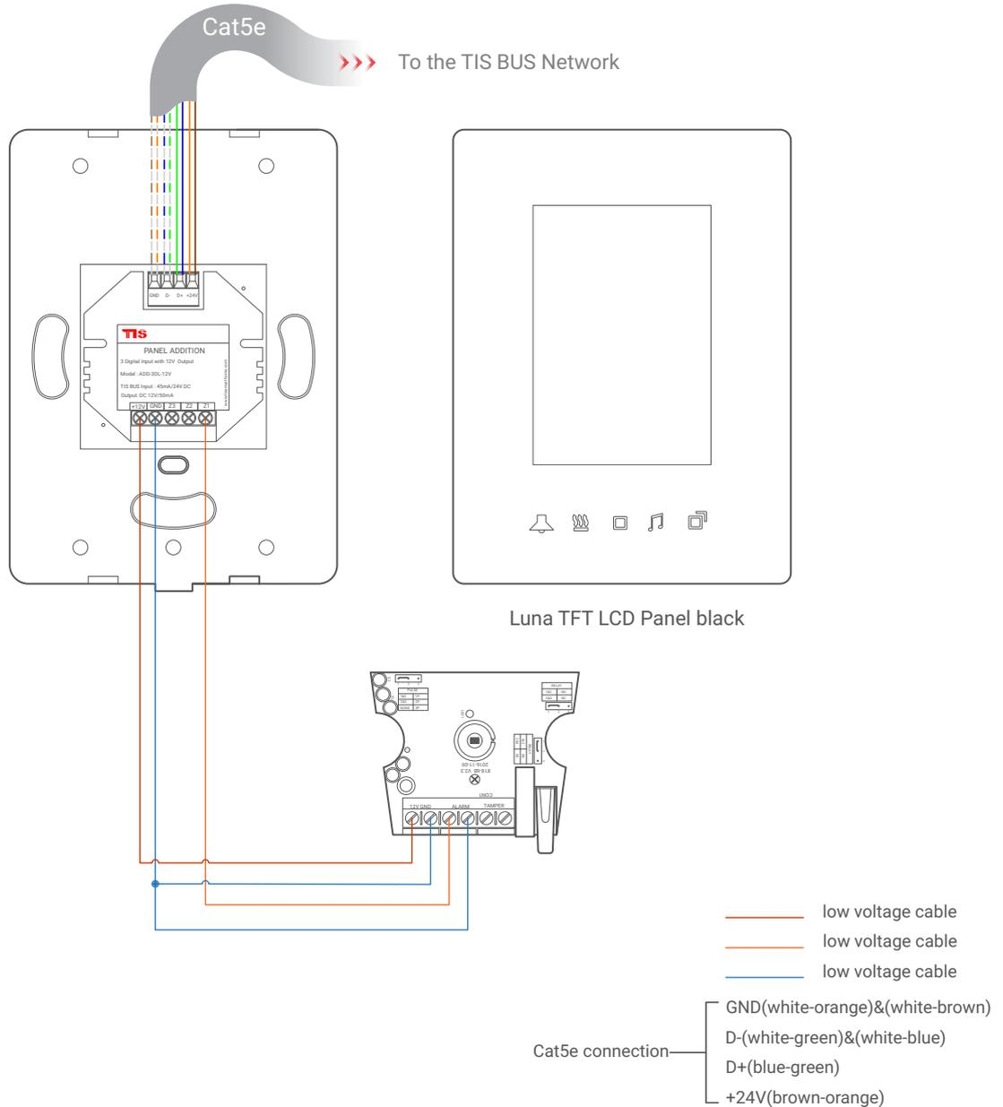
▲ Figure 6: Luna TFT & ADD-3DL-12V 3<sup>rd</sup> Party Sensor Connection Diagram
