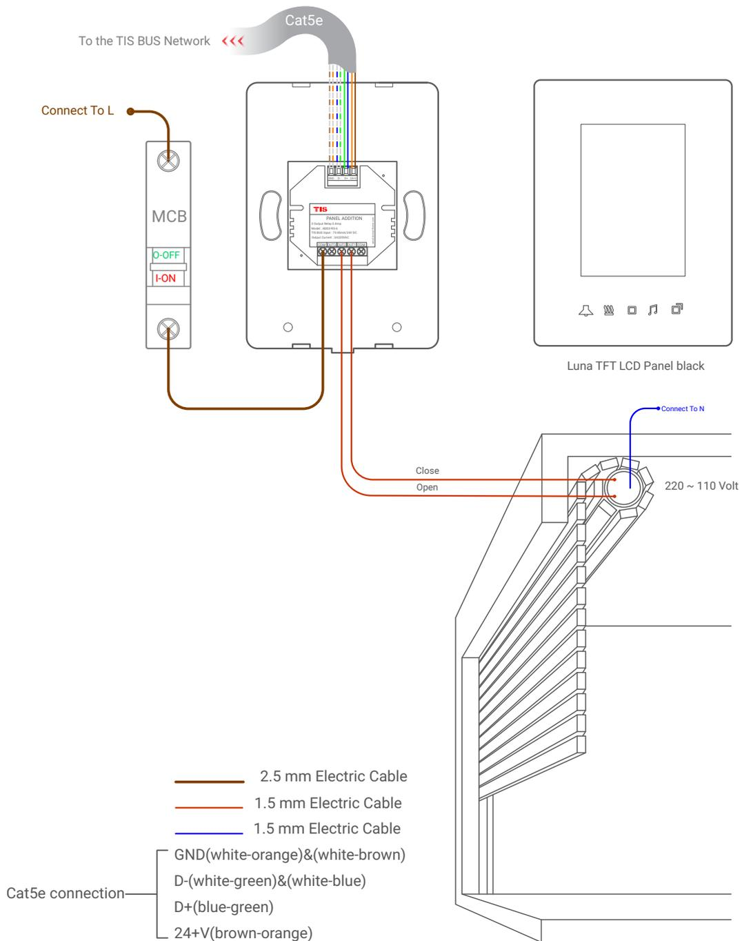
▲ Figure 3: Luna TFT & ADD-3R-5A Motors Connection Diagram
