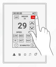
**3** Test your air conditioning by changing the mood, heat/cool, and fan speed from low to medium to high. The HVAC module should respond accordingly.
