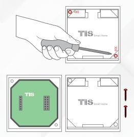
Addition in this position. Place the upper pins as shown, and then push the down pins down with your fingers to assemble.
