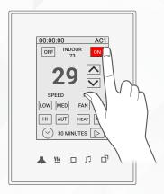
Test your air conditioning by changing the 3> fan speed from low to medium to high. Your relay should respond accordingly.
