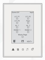
**6 >** The scene is programmed on the pressed button; you can test it with a single press.
