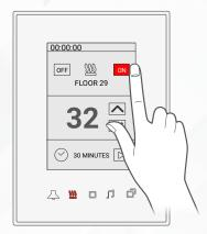
Test your floor heating by changing the 3> temperature; the relay should respond accordingly.
