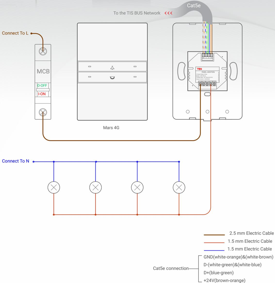
▲ Figure 1: Mars 4G & ADD-3R-5A Lights Connection Diagram
