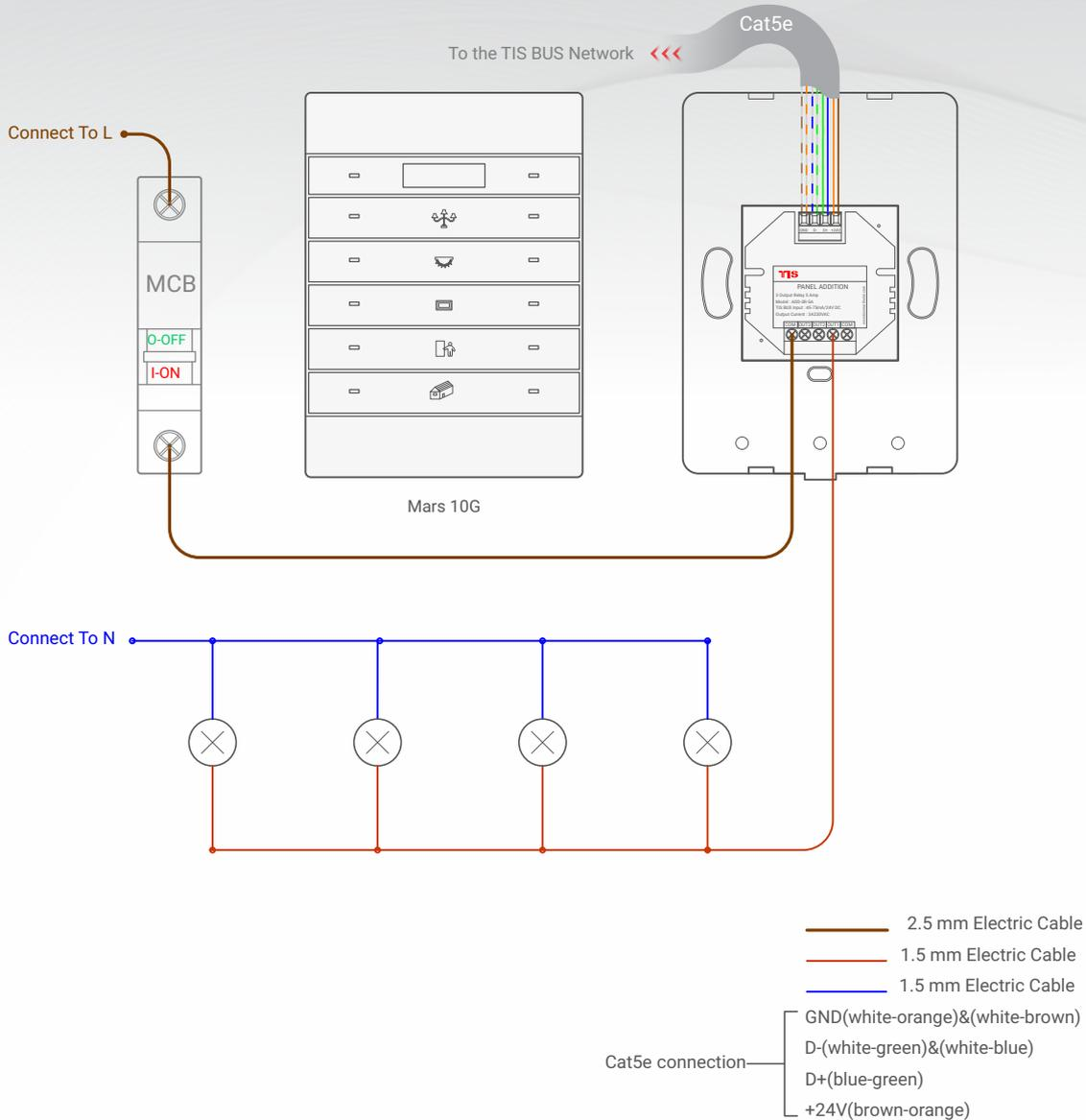
▲ Figure 1: Mars 10G & ADD-3R-5A Lights Connection Diagram
