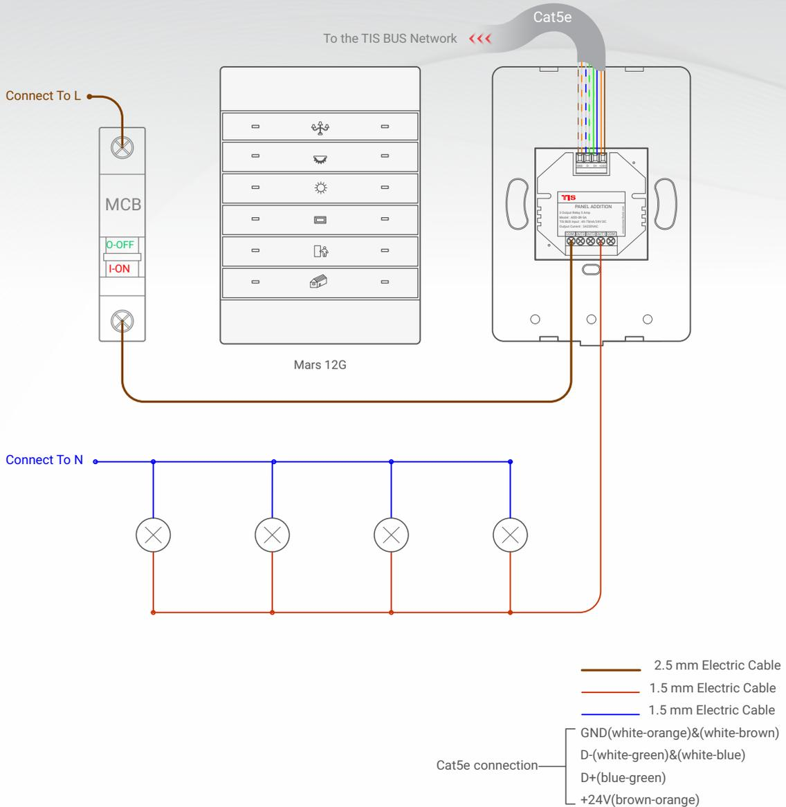
▲ Figure 1: Mars 12G & ADD-3R-5A Lights Connection Diagram
