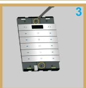
Remove the 2 black screws from the Mars Panel
