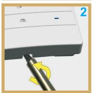
Rotate the screwdriver by 90 degrees.
