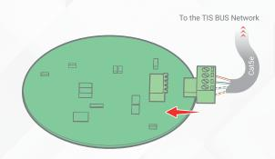
Secure the board inside the sensor base using the base pins.
