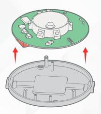
Open the wire holes, and insert the TIS-BUS cable in the sensor base.
