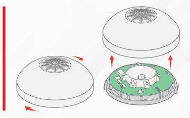
Remove the PCB from the holding pins.
