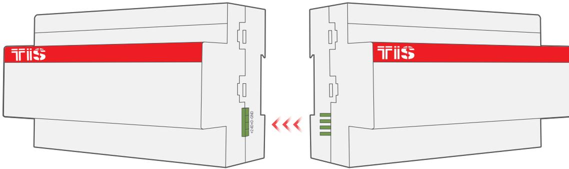
▲ Figure 5: DIN-Rail Bus Module Configuration Diagram
