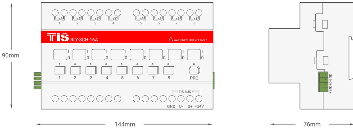
▲ Figure 6: Module's Dimension Diagram
