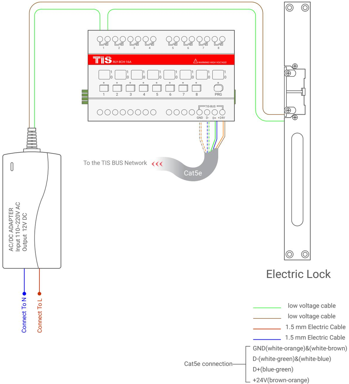
▲ Figure 3: Electric Lock Connection Diagram
