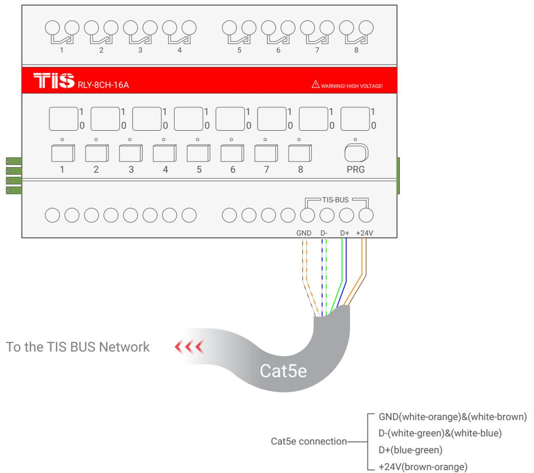
▲ Figure 4: Module's Bus Connection Color Coding
