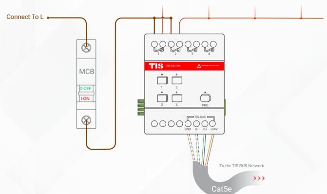
**6** Turn on the power source, and then test the loads by short pressing on the device's local override buttons 1-4.
