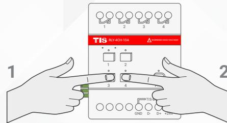
**3** » Wait for few seconds until the PRG LED stops blinking.
