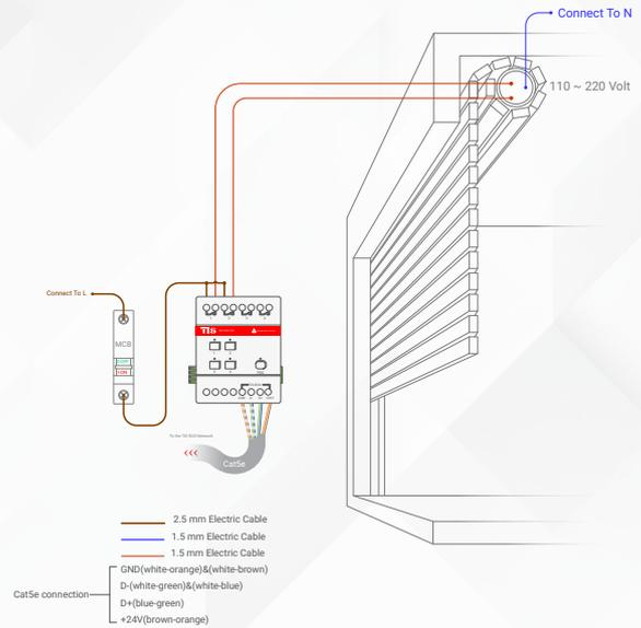
**5** Connect the live (supply) wire to inputs. All inputs must have an appropriate voltage source and an MCB to protect that load circuit.
