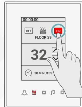
**3** Test the floor heating by changing the temperature and turning it OFF/ON.
