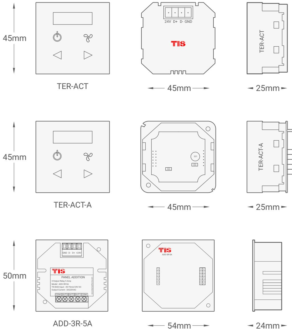
▲ Figure 8: Module's Dimension Diagram
