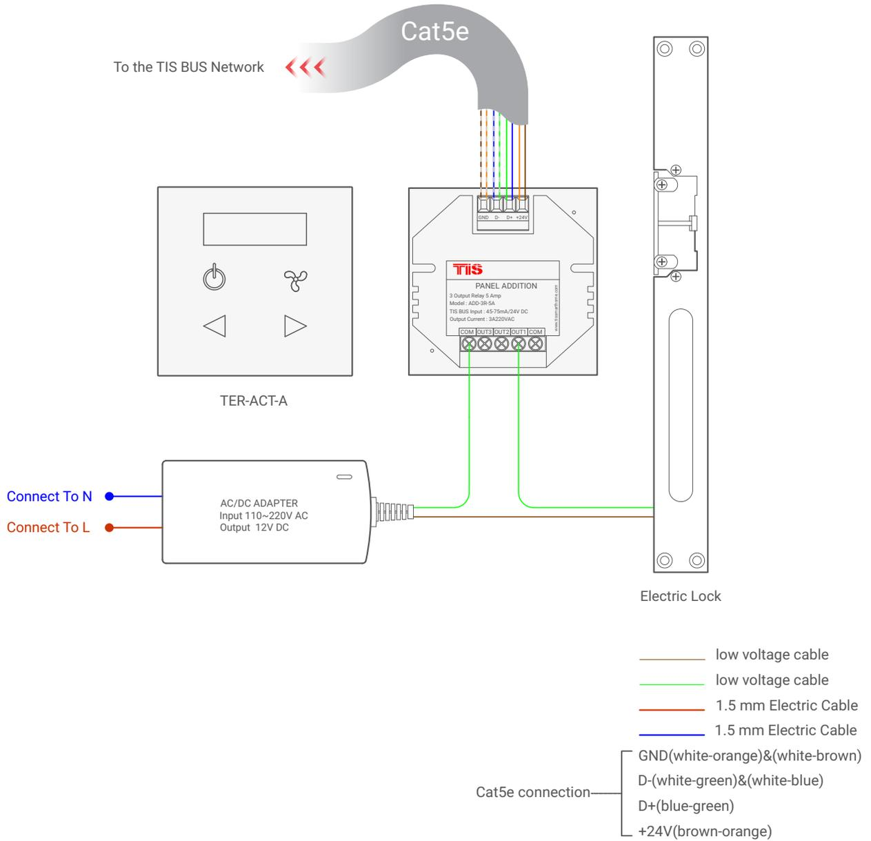
▲ Figure 4: TER-ACT-A & ADD-3R-5A Electric Lock Connection Diagram
