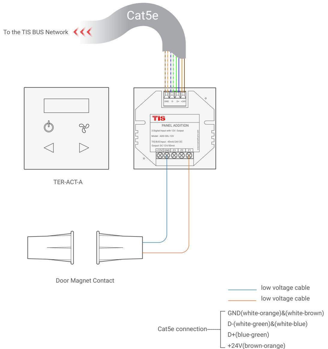
▲ Figure 5: TER-ACT-A & ADD-3DL-12V Magnetic Door Contact Connection Diagram
