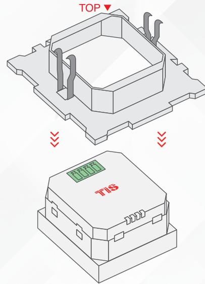
**3**» Connect the TIS-BUS Cable to the connector, and insert it into the Terre module.
