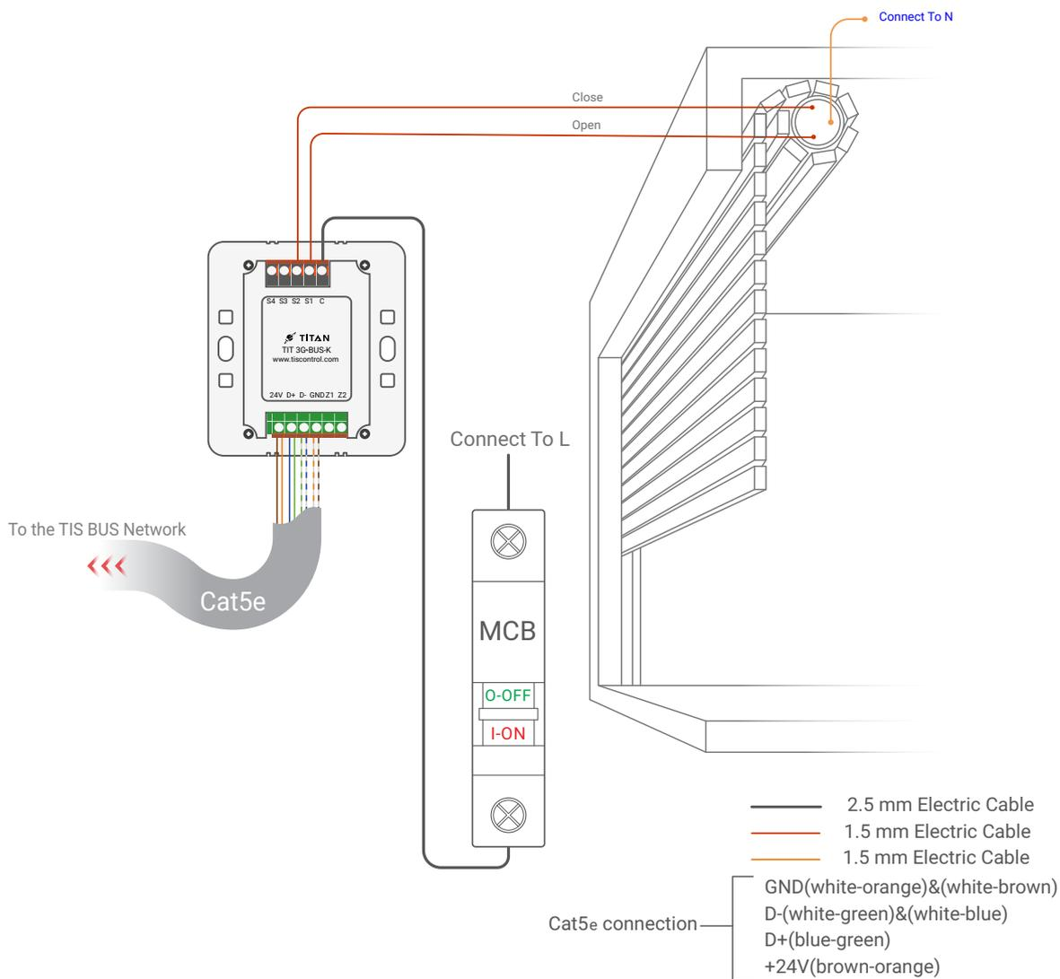
▲ Figure 2: TIT-3G-BUS-K & Motors Connection Diagram
