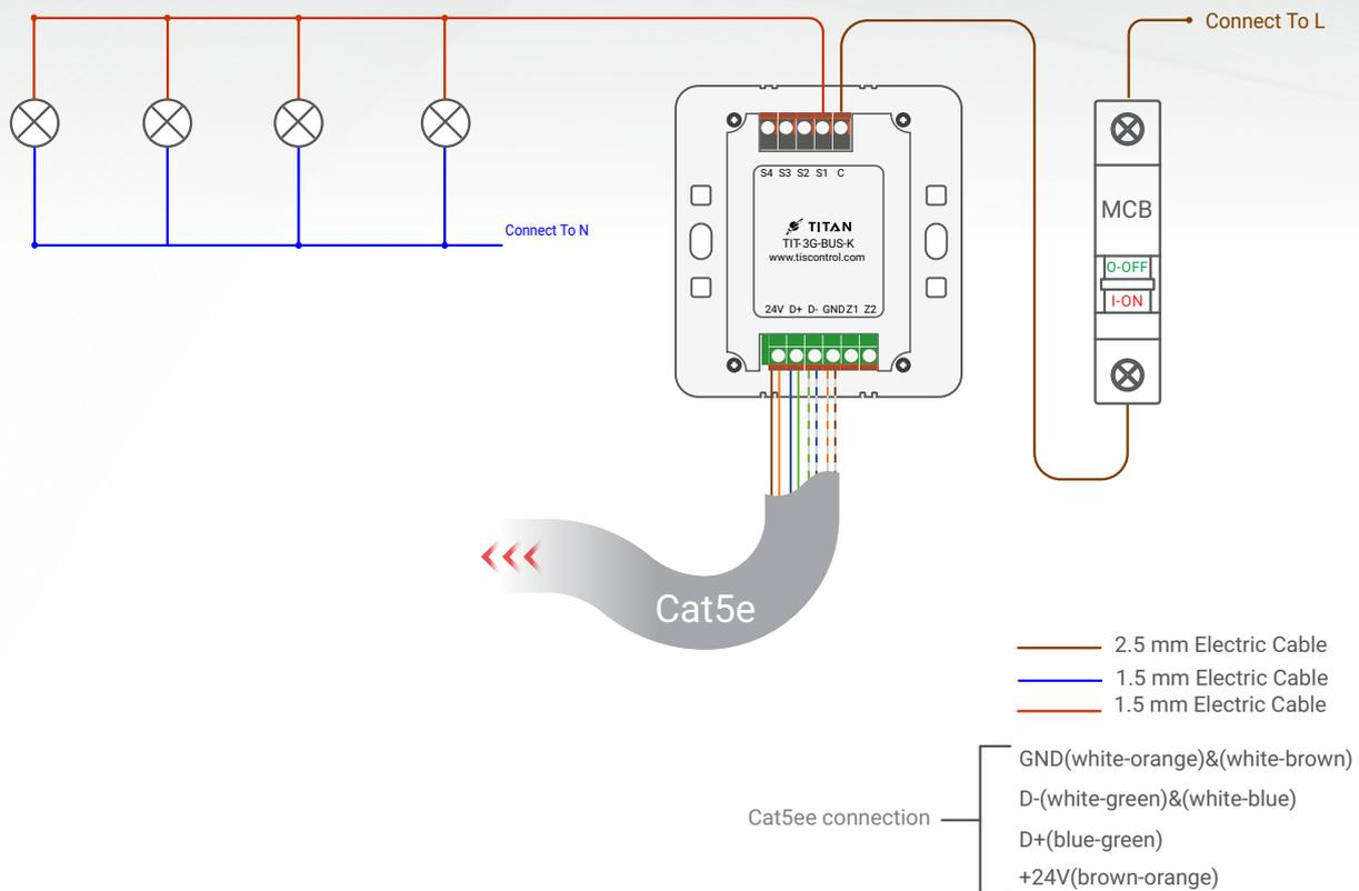
▲ Figure 1: TIT-3G-BUS-K & Lights Connection Diagram
