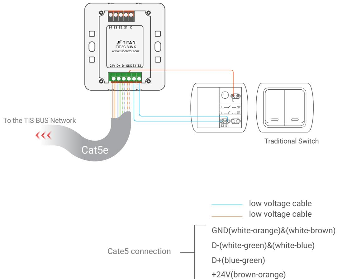
▲ Figure 5: TIT-3G-Bus-K & Traditional Switch Connection Diagram
