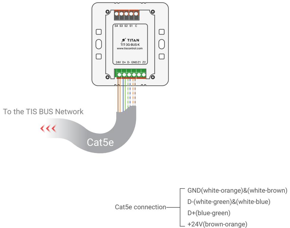
▲ Figure 6: TIT-3G-BUS-K Module's Bus Connection Color Coding
