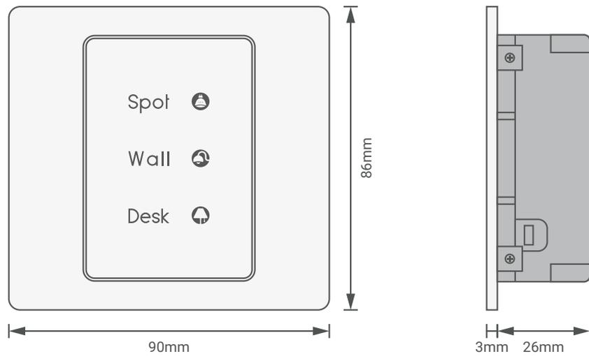
▲ Figure 7: TIT-3G-Bus-K Module's Dimension Diagram
