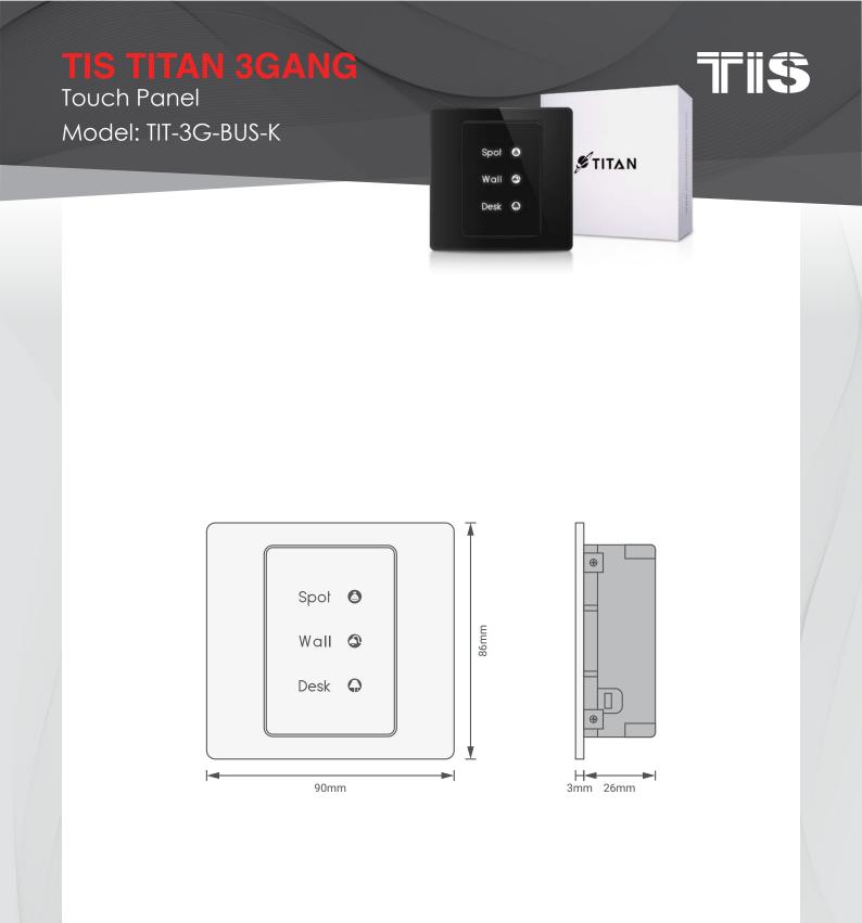
Figure 7: TIT-3G-Bus-K Module's Dimension Diagram
