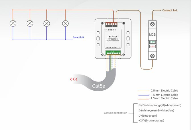
Figure 1: TIT-3G-BUS-K & Lights Connection Diagram
