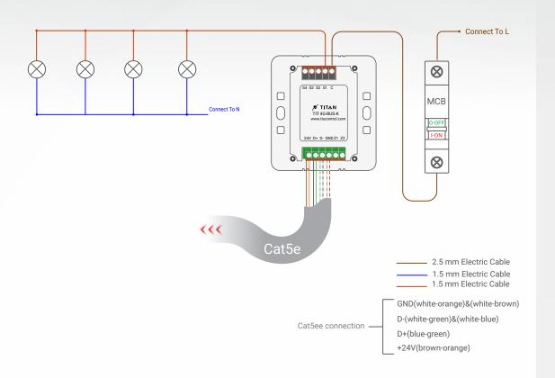
Figure 1: TIT-4G-BUS-K & Lights Connection Diagram
