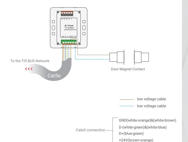
Figure 3: TIT-4G-BUS-K & Magnetic Door Contact Connection Diagram
