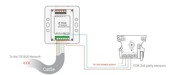
low voltage cable low voltage cable low voltage cable low voltage cable GND(white-orange)&(white-brown) D-(white-green)&(white-blue) Cate5 connection -D+(blue-green) +24V(brown-orange)
