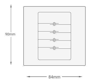
Figure 7: TIT-4G-Bus-K Malule's Dimension Diagram
