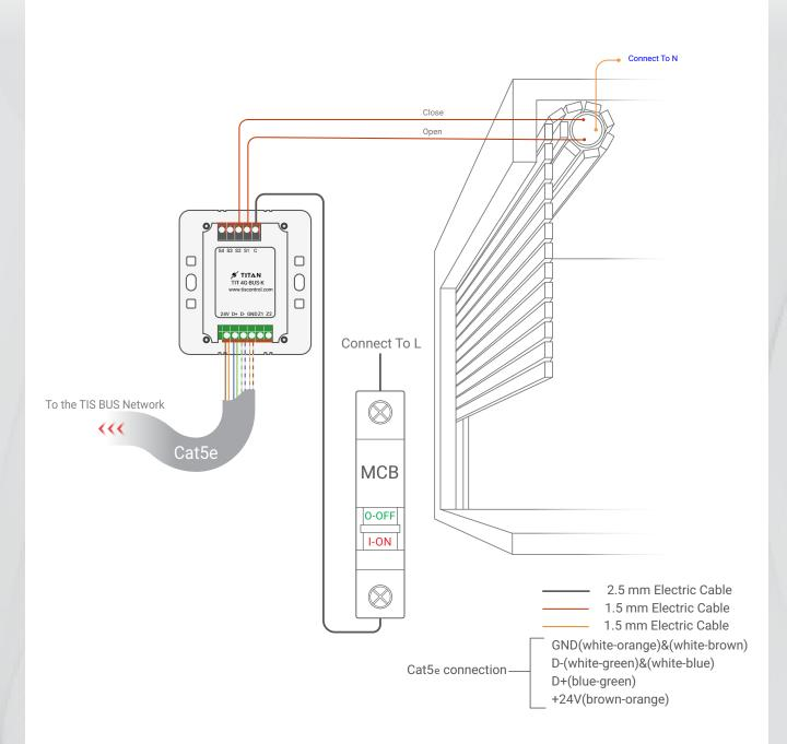
Figure 2: TIT-4G-BUS-K & Motors Connection Diagram
