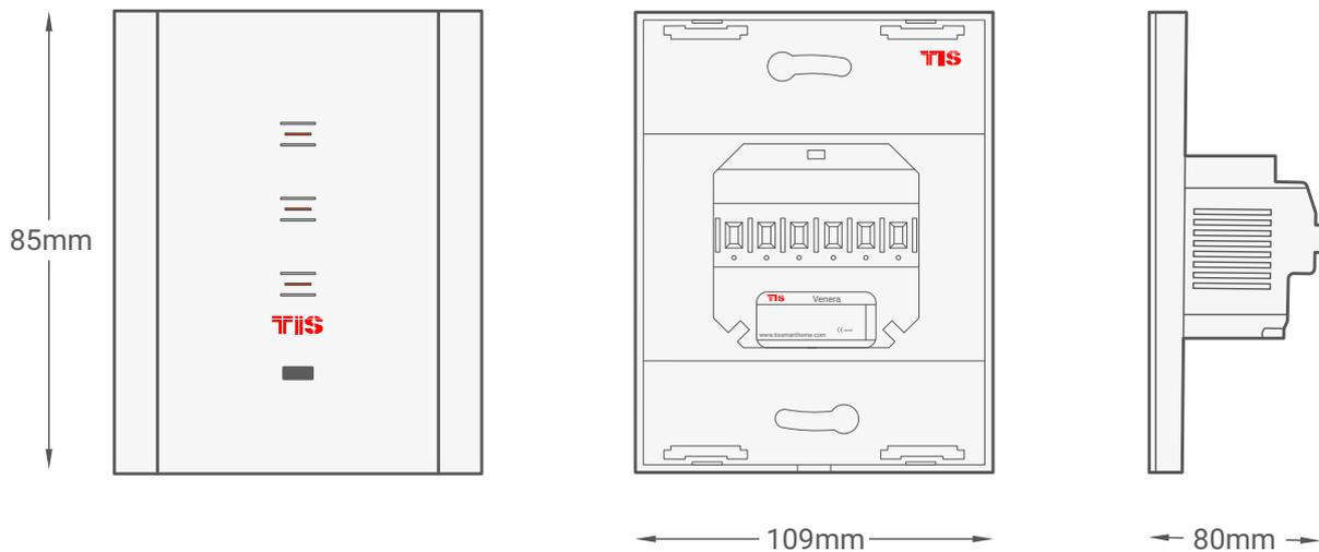
▲ Figure 4: Module's Dimension Diagram
