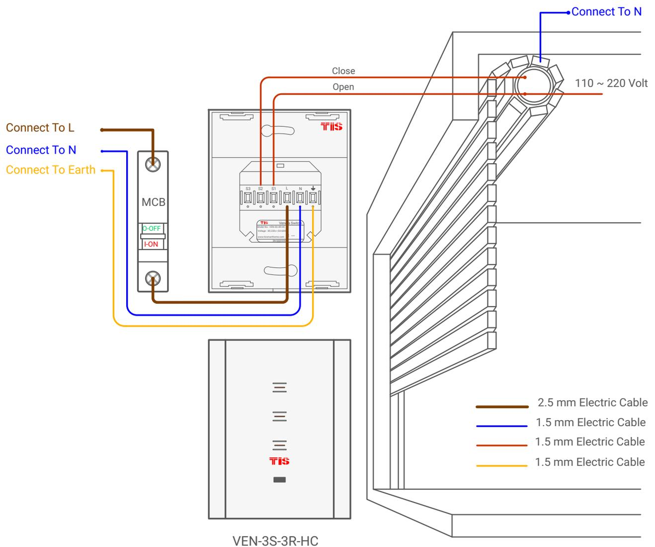
▲ Figure 2: VEN-3S-3R-HC Motors Connection Diagram
