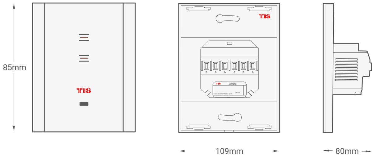
▲ Figure 3: Module's Dimension Diagram
