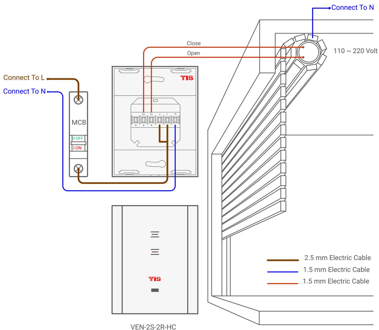
▲ Figure 2: VEN-2S-2R-HC Motors Connection Diagram
