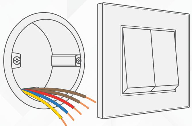
**3** There should be a total of 3-5 wires (3 wires if 1 gang, 4 wires if 2 gangs, 5 wires if 3 gangs). Find the neutral wire.
