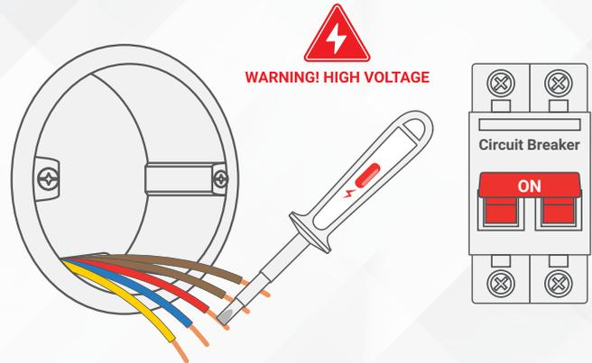
**5** Turn off the power at the main power breaker again to turn off the voltage supply to the switch.
