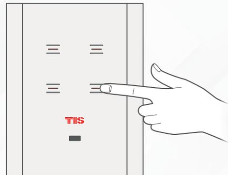
**3** Test the button on the panel by short pressing it for ON/OFF and long pressing to dim.
