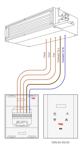
2.5 mm Electric Cable 1.5 mm Electric Cable 1.5 mm Electric Cable
