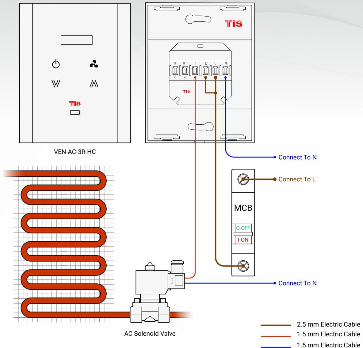
▲ Figure 1: VEN-AC-3R Floor Heating System Connection Diagram
