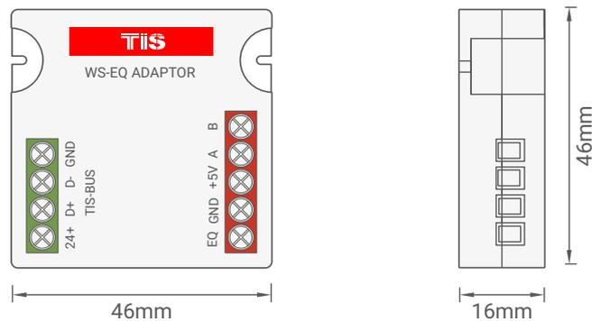
▲ Figure 2: WS-EQ ADAPTOR Module's Dimensions
